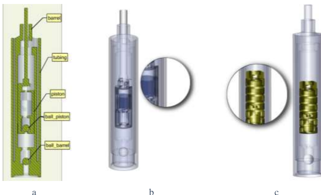
Figure 1. The main elements of a borehole pump: a. a section through the pump; b. a polished piston; c. a piston with ditches.
