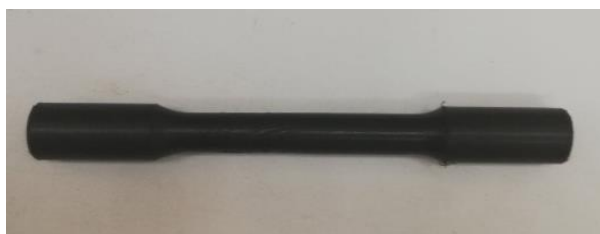
Figure 4. The specimen test taken to be subjected to the application of rotating-bending test
