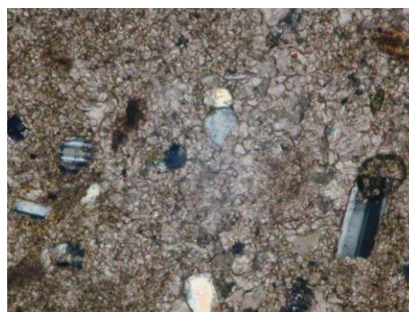
Fig. 8. Microphotograph. Dolomicrosparite with quartz and plagioclase feldspar. N(+) x10.
