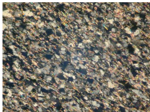
Fig. 22. Microphotograph. Epimetamorphic rock (quartzitic-micaceous schists) from the series of the green schists. N(+), x25.
