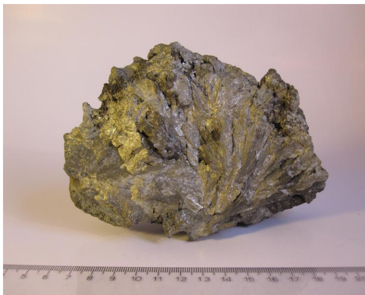
Fig.1. Polymetallic sample with iron sulphides (pyrite and marcasite) from Herja ore deposit
