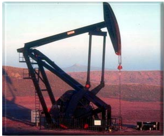
Fig. 1. Reverse schematic pumping unit
