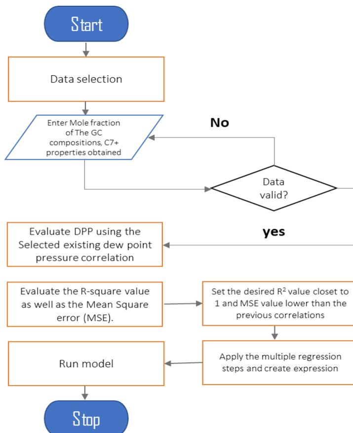
Figure 2: Process flowchart showing the procedures for the data analysis
