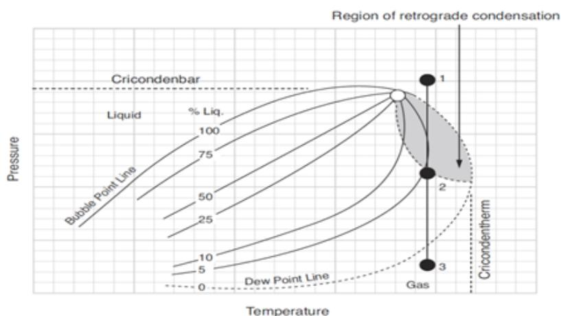
Figure 1. Gas condensate reservoir's Phase Diagram displays Retrograde Condensation conditions [2]
