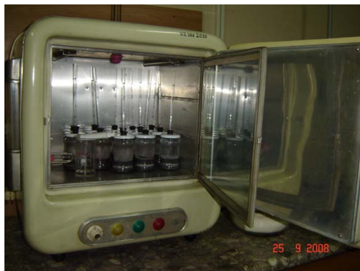
Fig. 4. Measuring the chemical shrinkage through the dilatometric method.
