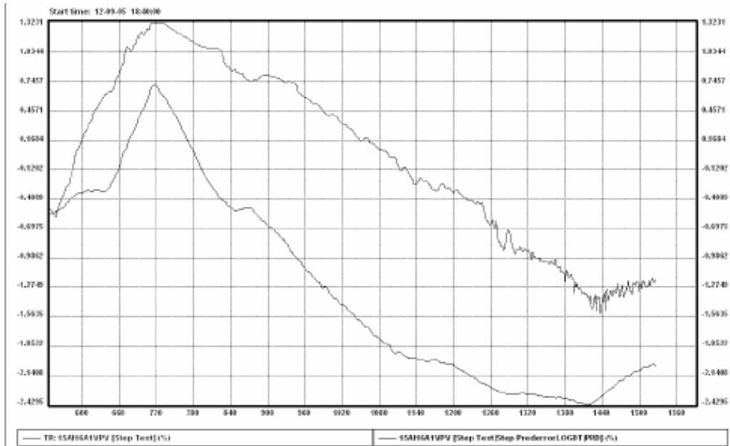
**Fig. 8.** Predicted and obtained impurities within bottom product (top graph dynamic simulation prediction, bottom graph real process value after DMC model implementation)
