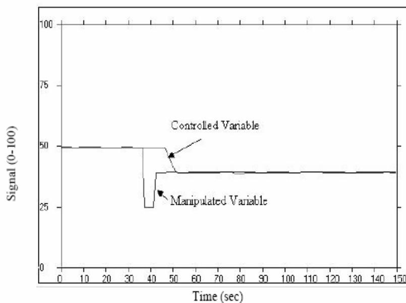
**Fig.7.** Demonstration of DMC control
