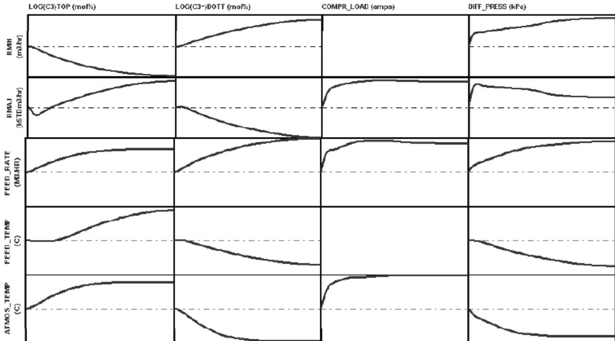
Fig.6. Dynamic matrix generated by using step test data
