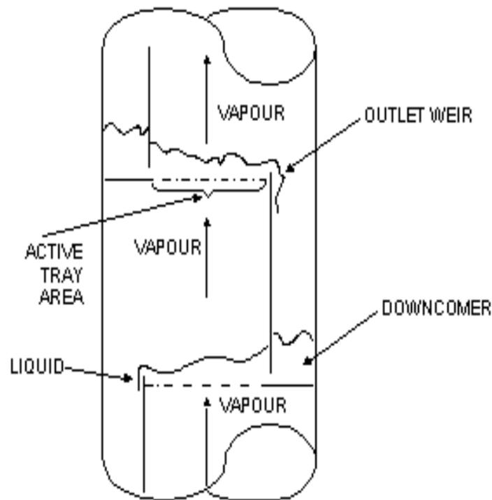
**Fig. 3** Distillation column liquid holds up
