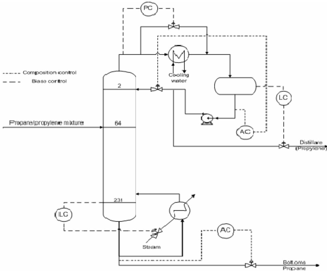
Fig. 1. The Superfractionator (C3 Splitter) with its base control system
