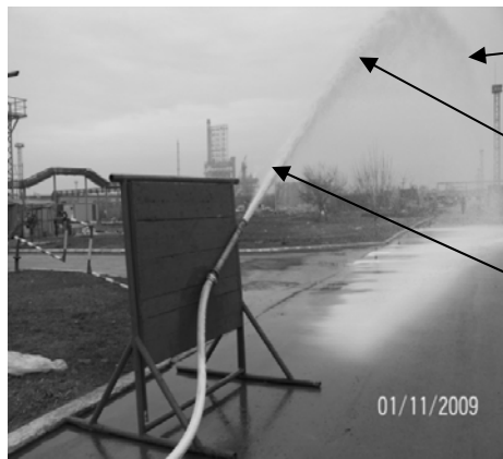
Fig. 8. Jet's structure at a 5000 l/min foam
