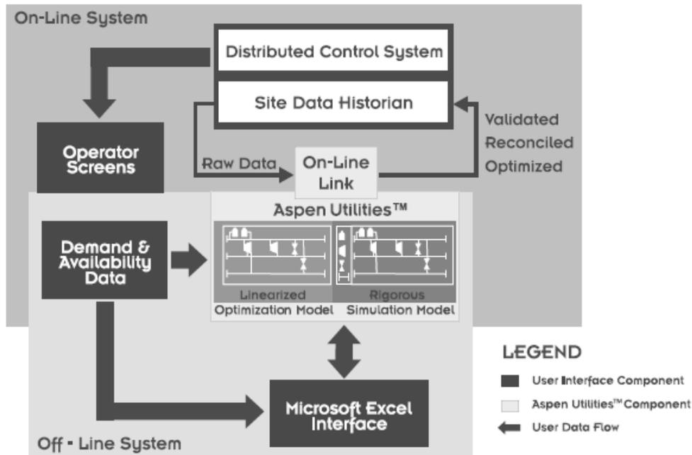
**Fig. 1** Refinery energy savings control structure
