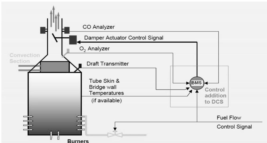
**Fig. 2.** Proposed excess air control diagram
