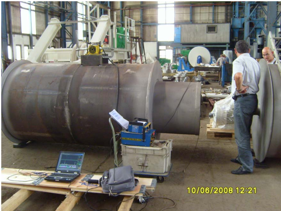
Fig. 6. Evaluation of Meta-Lax VSR treatment; our laptop with spectrum analyzer software (bottom)
