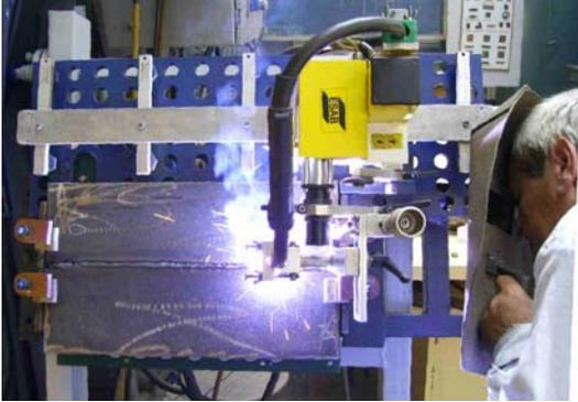
**Fig. 3.** Horizontal position on a vertical wall-cornice (PC) MAG - C mechanized welding of the samples [4]
