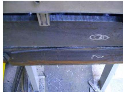
**Fig. 5.** The easy separation of slag on horizontal position on a vertical wall-cornice (PC) MAG - C mechanized welding [3, 4]
