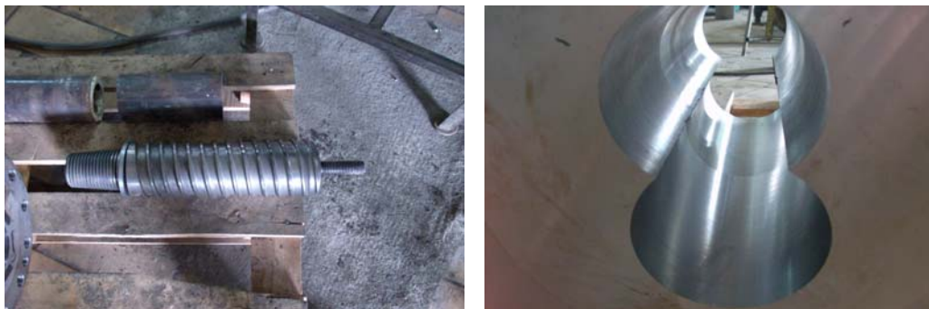
a. b. Fig. 1. Products subjected to reconditioning: a. worm gear; b. stator
