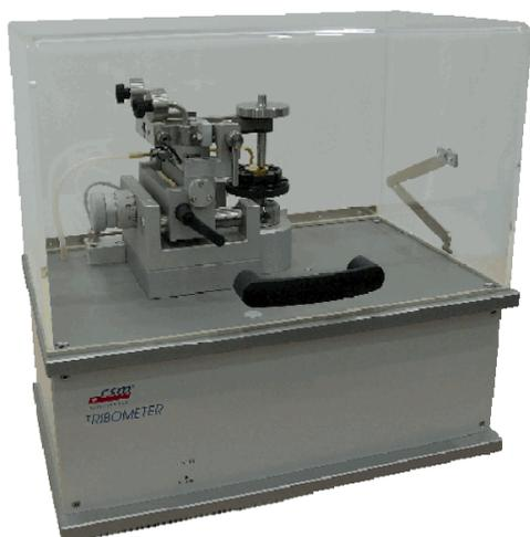
**Fig. 5.** The C.S.M. tribometer
