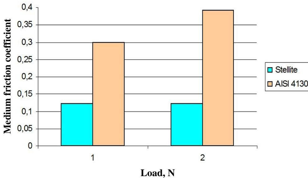
Fig. 9. Schematic representation of the average friction coefficient, depending on load
