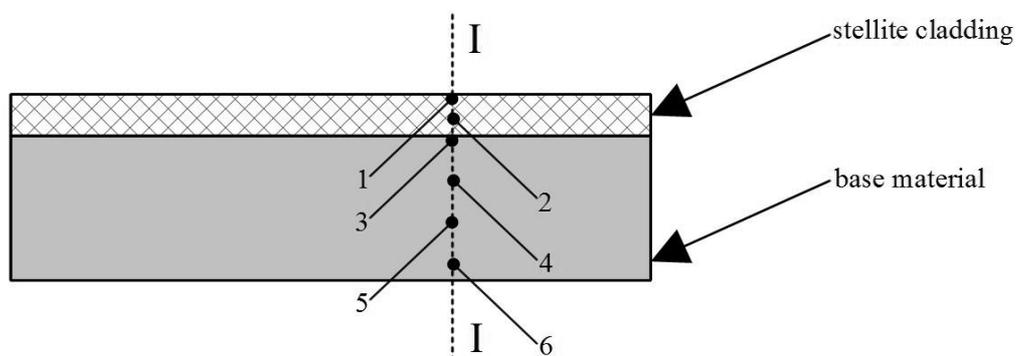
**Fig. 4.** Hardness measurement locations on the samples cladded using the MIG procedure
