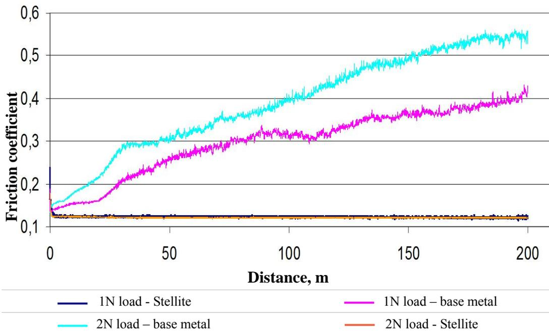
Fig. 8. Friction coefficient variation, depending on distance for loads of 1N and 2N
