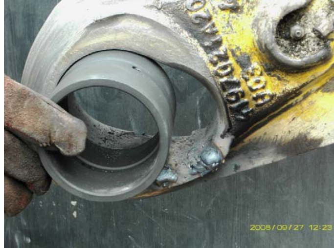
Fig. 7. Renewall the bore of the main arm of a loader
