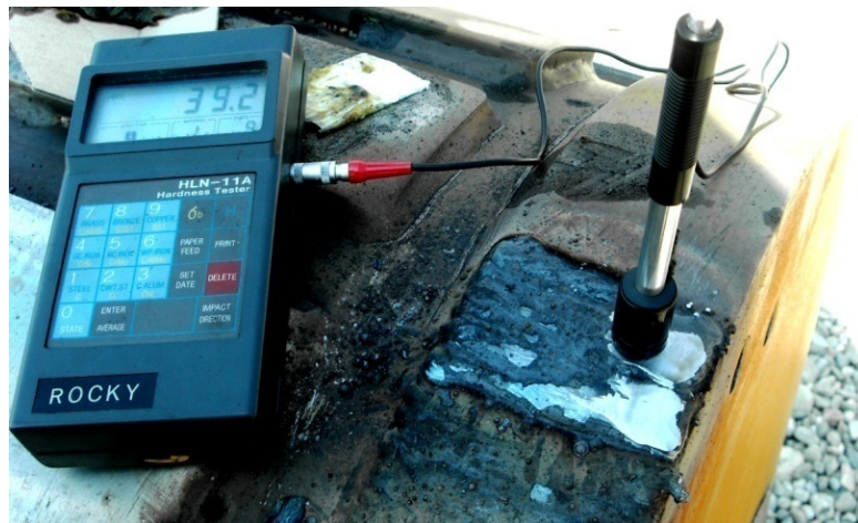
Fig. 13. Hardness testing after built-up welding
