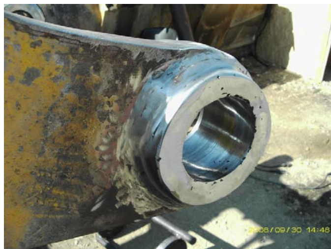
Fig. 8. Renewall after repairing by welding and adjusting
