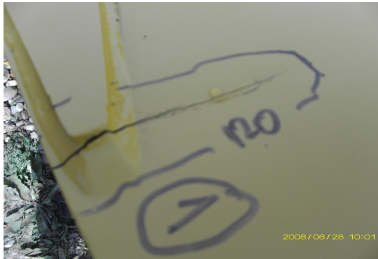
Fig. 1. Visual testing showing a crack on excavator arm
