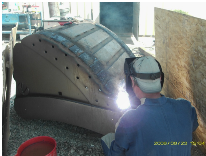
Fig.12: Built-up welding on bucket wear plates
