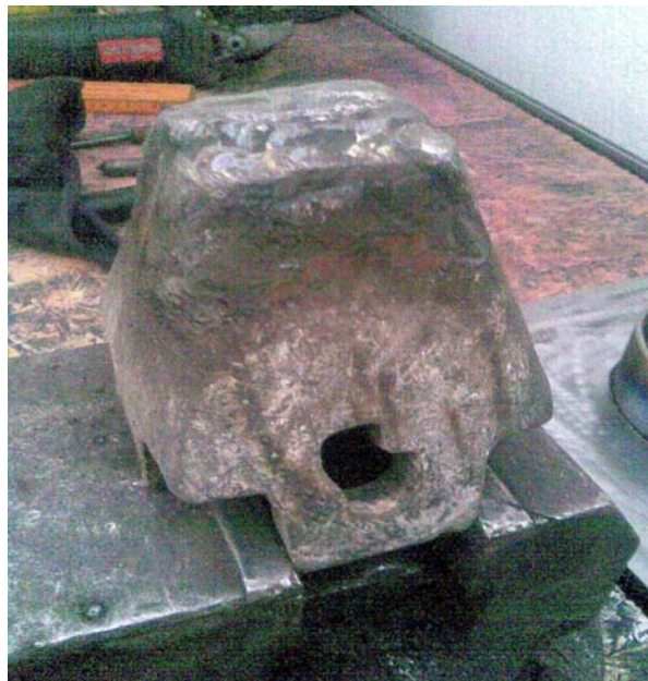
Fig. 14. Bucket tooth repaired by welding (hardfacing)
