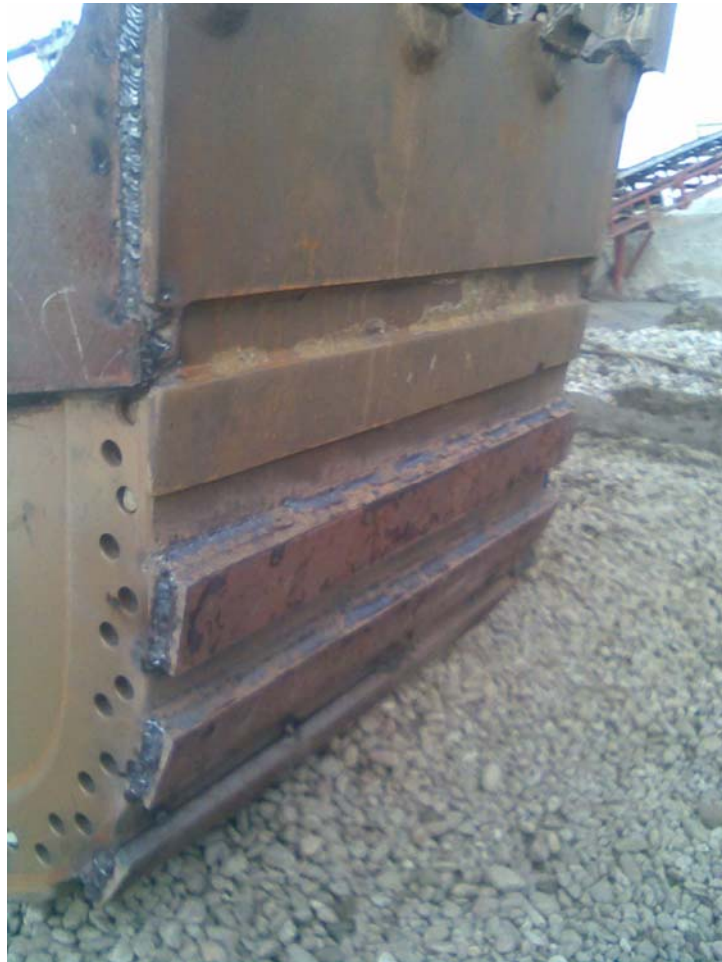
Fig. 15. Excavator bucket rehabilitated using HARDOX wear plates
