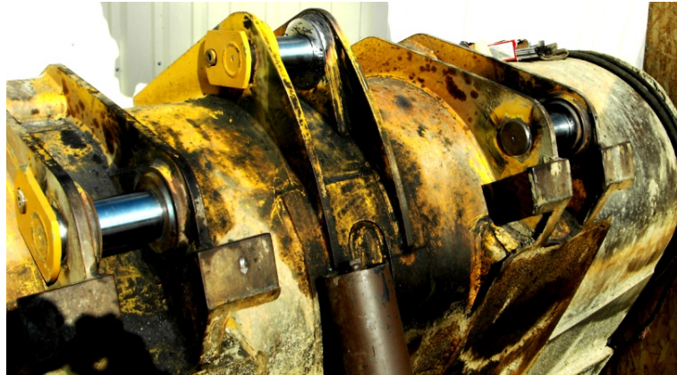
Fig. 11. Rehabilitated bores by welding and adjusting
