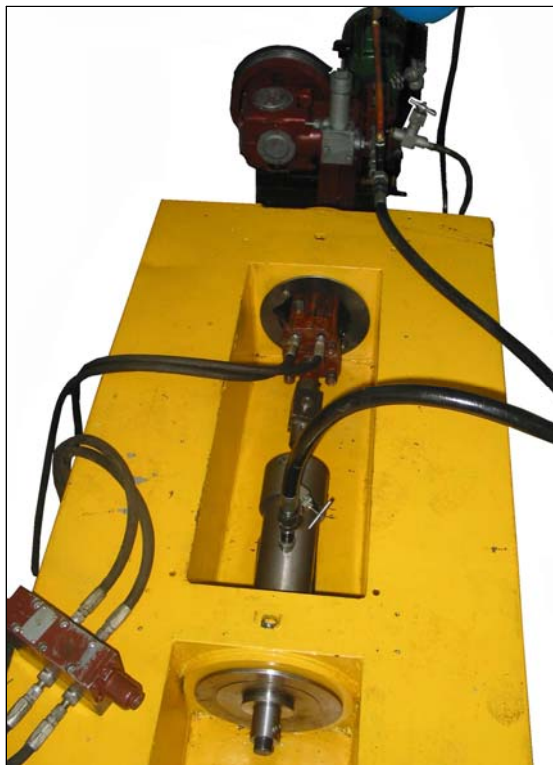
Fig. 2. The general view of the testing facility to external pressure (collapse) and axial tension.
