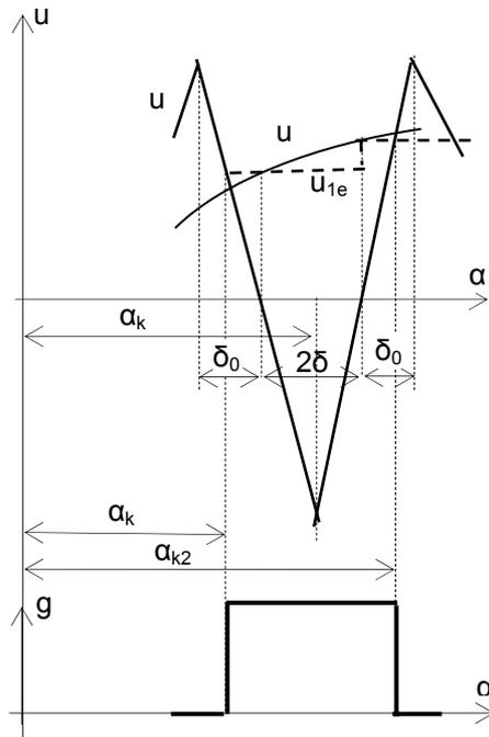
Fig.4. Principle of sine-delta PWM sampling modulation
