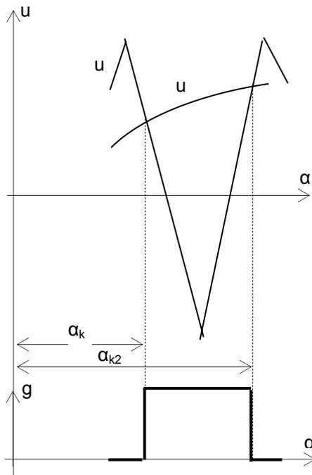
**Fig.2.** Principle of sine-delta PWM natural modulation.
