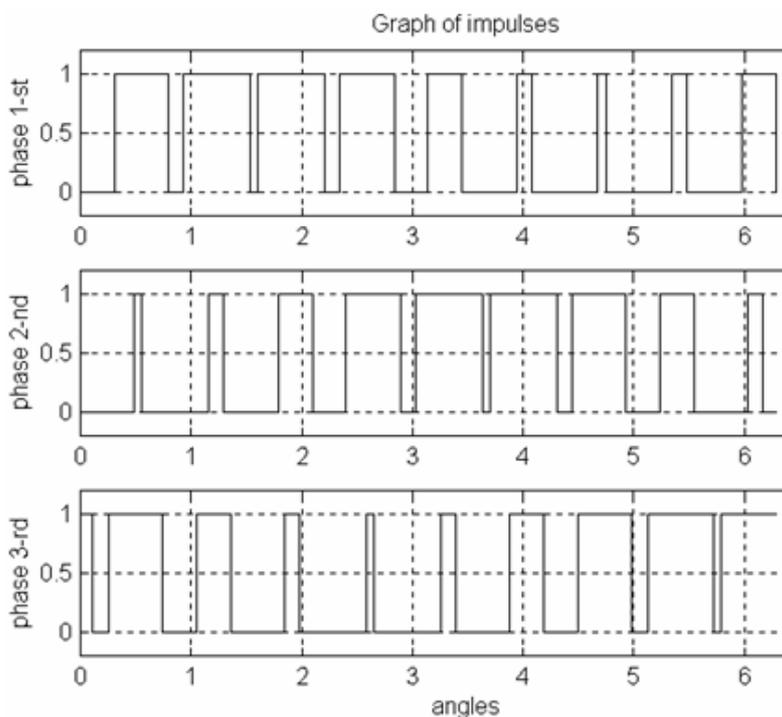
Fig. 5. The waveform of command impulses obtained by simulation
