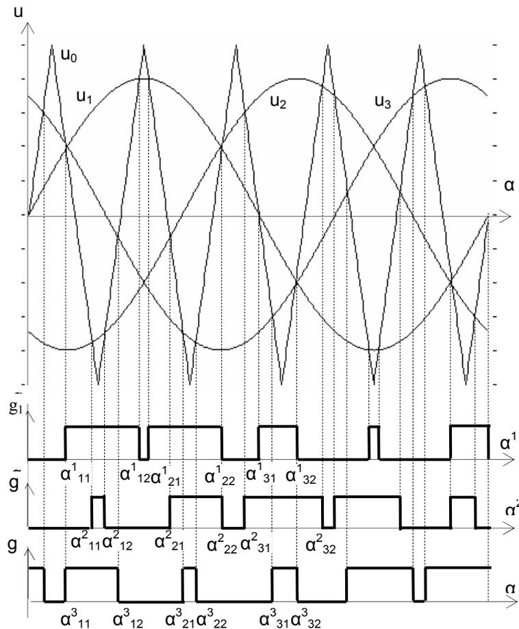
**Fig. 3.** The impulses of sine-delta PWM natural modulation
