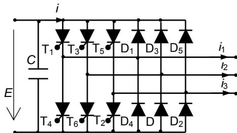
**Fig. 1.** The electric scheme of voltage three-phase
