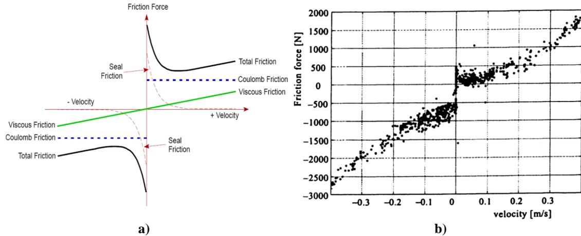
**Fig. 2.** Friction force in a linear actuator:
