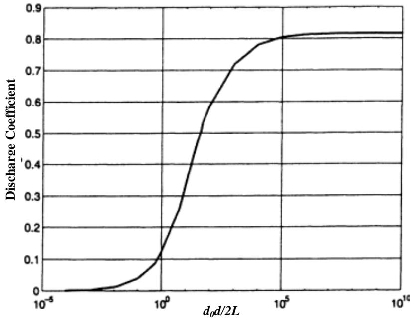
Fig. 1. Discharge coefficient  $\alpha_d$  for orifices [5].
