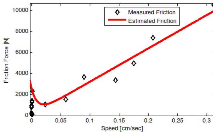
**Fig. 4.** Measured and approximated friction force for a big single-acting hydraulic cylinder.
