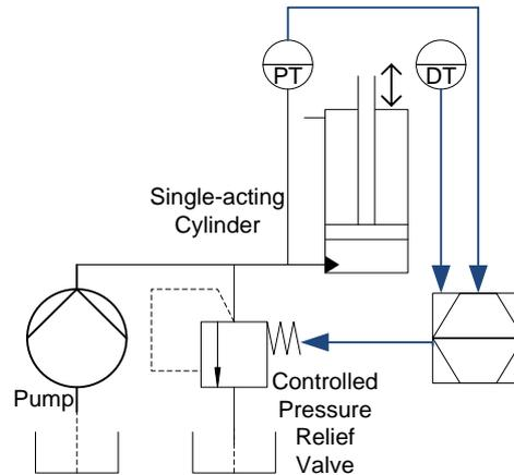
**Fig. 3.** The schematic of the friction measurement system.
