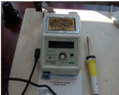
Fig. 2. Heat source to eutectic solder
