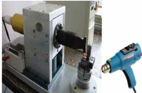
Fig. 3. Used installation in thermo sonic micro- joining
