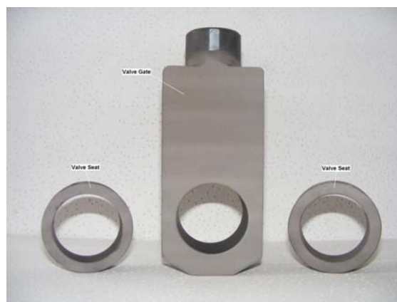
Fig.4. Valve seat and valve gate hardfaced with tungsten carbide by using the HVOF process.
