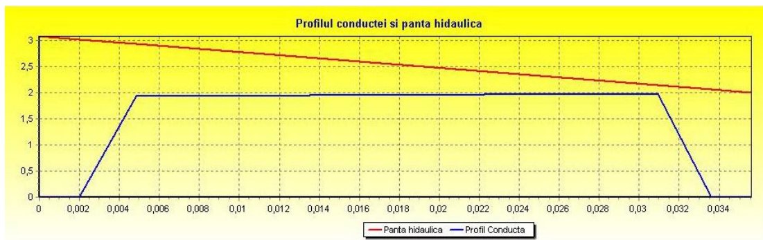
Fig. 7. L1 Hydraulic slope and Pipeline profile
