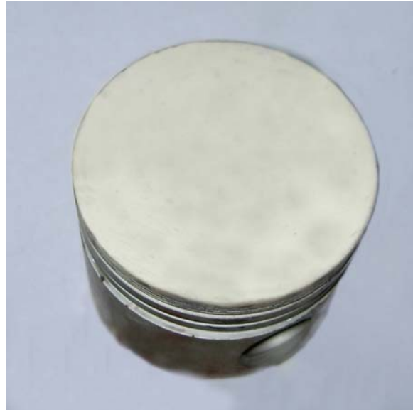
Fig. 1. Piston with ceramic crown
