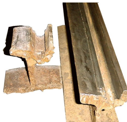
Fig. 6. A worn out rail, before reconditioning and one after reconditioning
