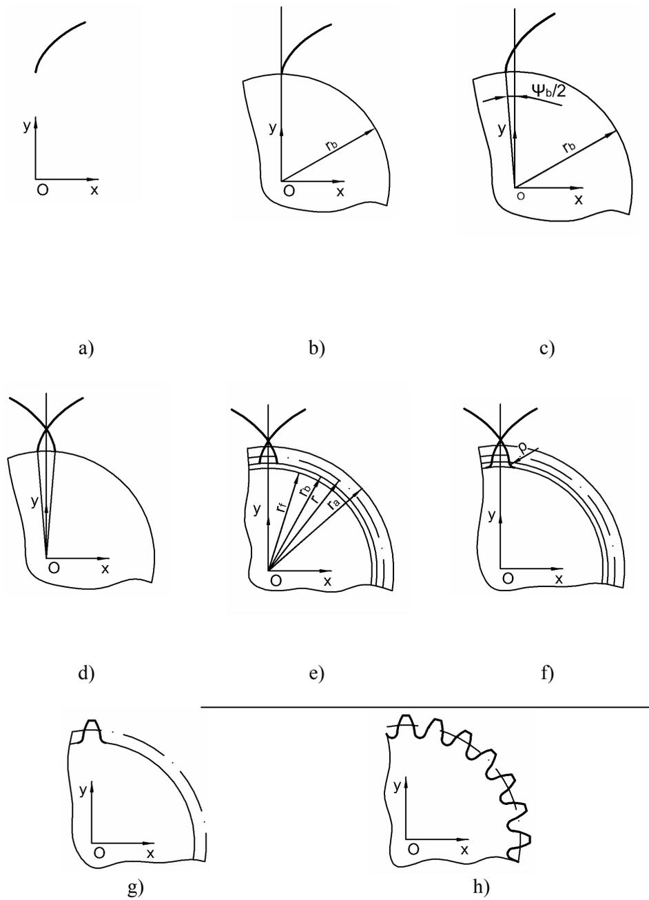
**Fig. 3.** The steps for gear's teeth engendering:
