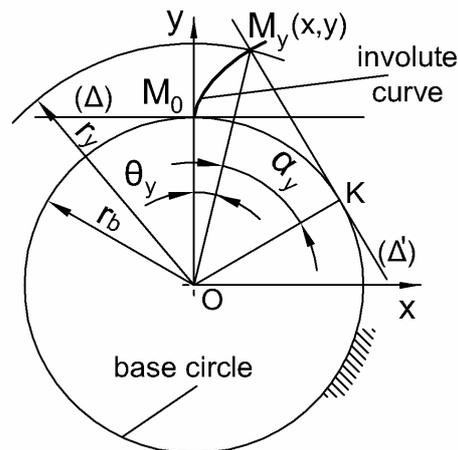
**Fig. 1.** Engendering the involute curve
