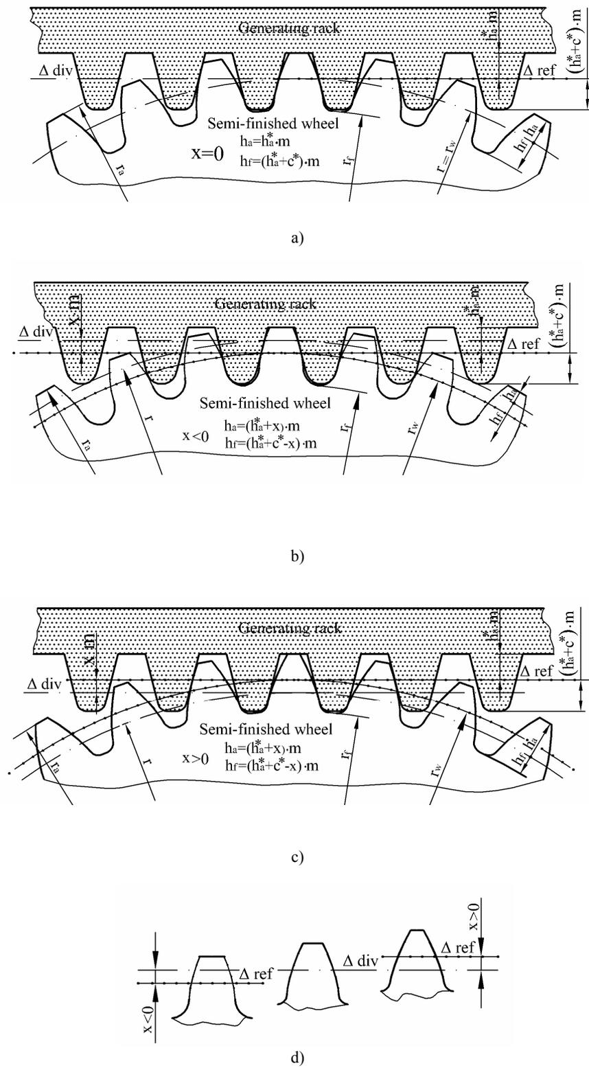
Fig. 4. Aspects regarding the gear's engendering with profile correction".
