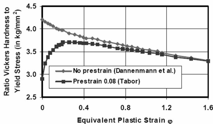
Fig. 2: Ratio of Vickers Hardness Number and Yield Stress, by Dannenmann and Wilhelm [1]
