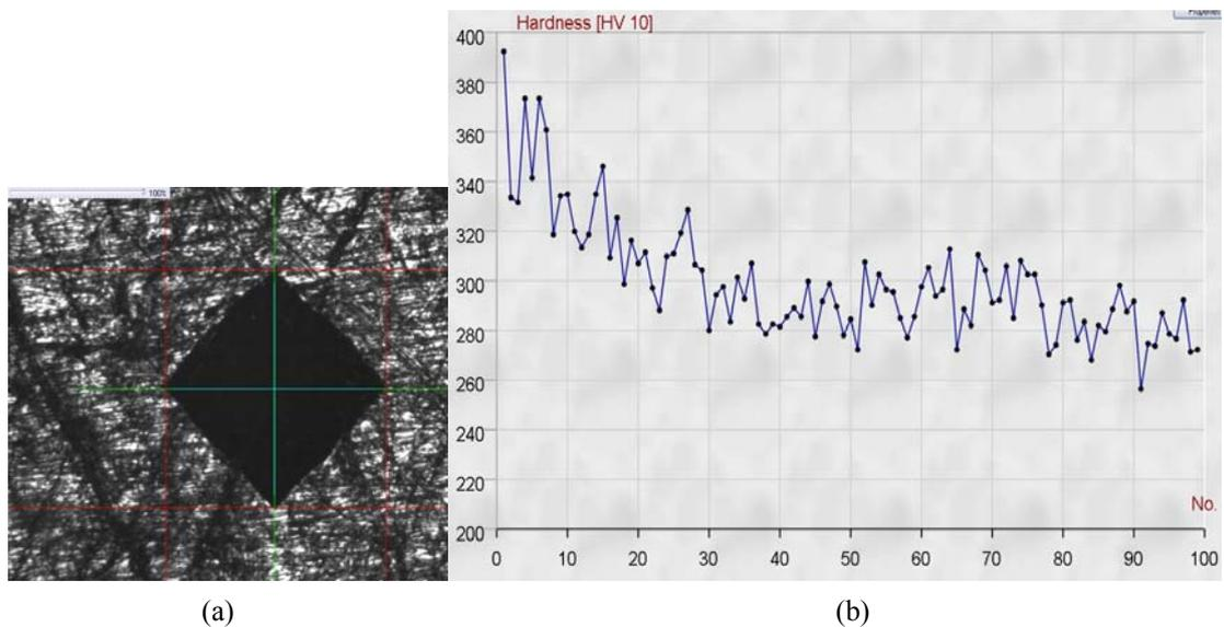
Fig. 6. a) The imprint of Vickers indenter; b) Vickers micro hardness values.
