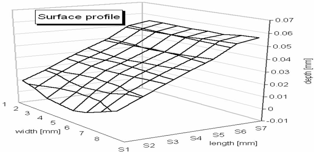
Fig. 5. The surface profile into the vicinity of the fracture section.
