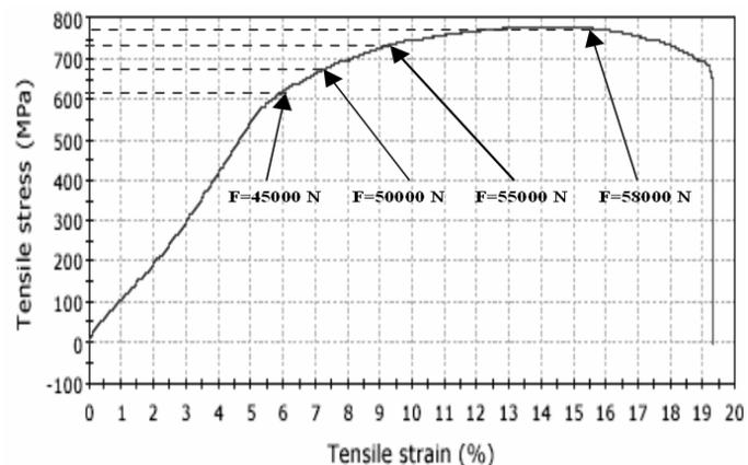
**Fig. 4.** Typical stress-strain dependence for studied alloy steel.
