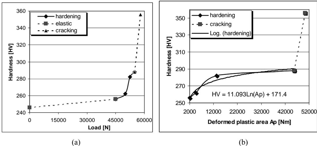
Fig. 9. a) Hardness - load dependence; b) Hardness - plastic area dependence.
