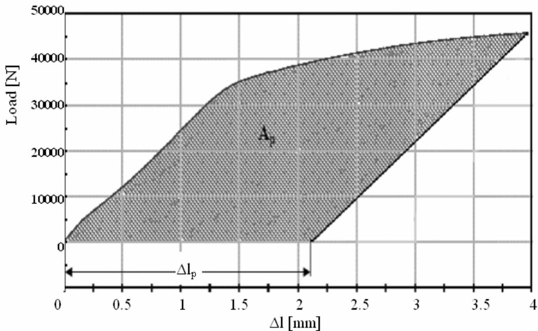
**Fig. 8.** The area ( $A_p$ ) of the plastic strain domain.
