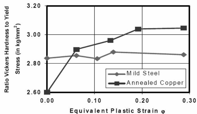
Fig. 1: Experimentally determined Vickers Hardness Number and Yield Stress ratios for various amounts of initial plastic strain [6]
