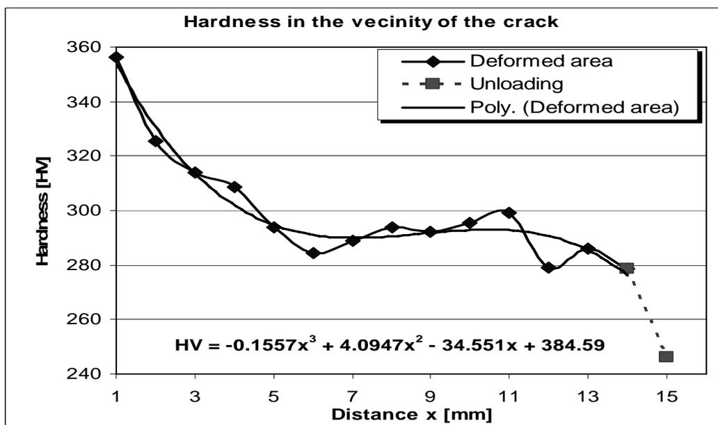
**Fig. 7.** Micro hardness values in dependence with the distance from the crack.
