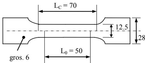
**Fig. 3.** Typical shape of tension test specimen
