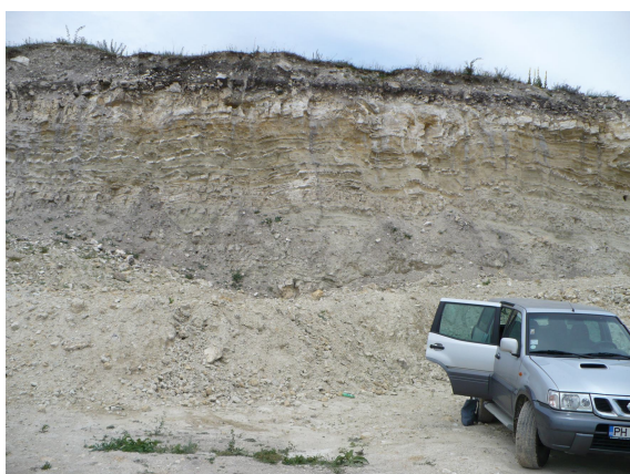
Fig. 6. View of the superior slope of the quarry with an interval of about 8m of transition of sandy layers with subdecimetric intercalations of lumachellic limestone, situated between the lower and the upper bank of Istrița limestone
