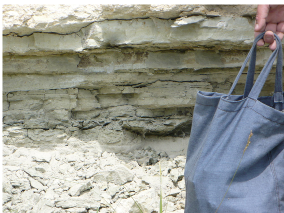
Fig. 4. Tuffaceous arenite in the basis of slope 1 of the Istrița limestone quarry from Năeni
