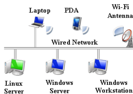
Fig. 4. Typical control network infrastructure.
