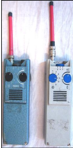
Fig. 9. RTP-4MF-S military-type radio transmitters.
