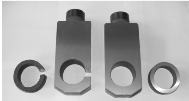
Fig. 2. Specimens hardfaced with tungsten carbide machined by grinding
