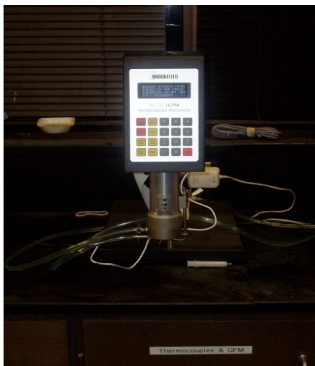
Fig. 3. Picture showing the experimental setup of Brookfield viscometer
