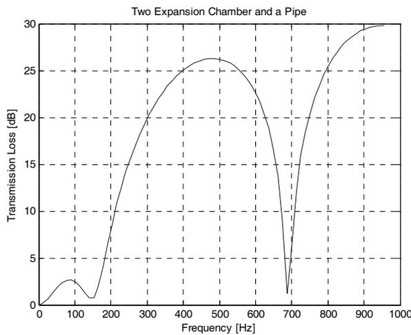
Fig. 4. Transmisson loss, relation 14, for the attenuator represented in figure 2.
