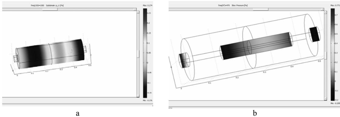
Fig. 7. Distribution of acoustic pressure in the elements of attenuator.
