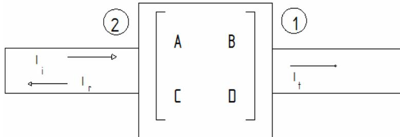
Fig. 3. Elements used to define transmission loss.
