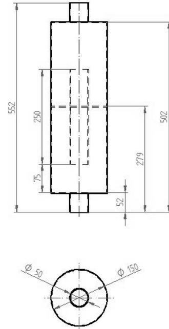
Fig. 2. A model for a reactive attenuator.
