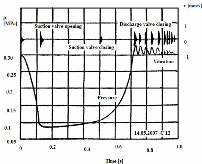
Fig. 8. A source of vibration induced by springs of discharge valve.
