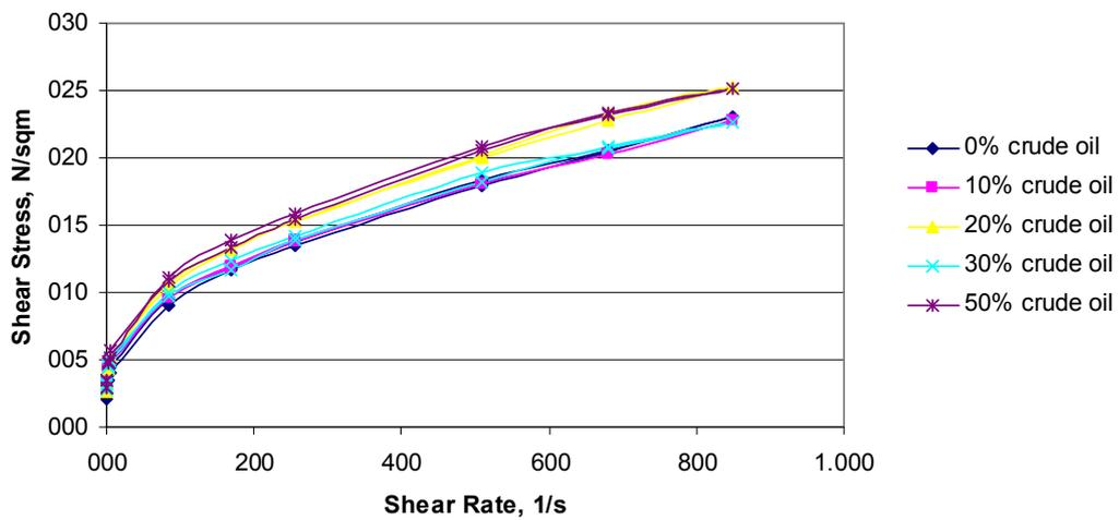
Fig. 8. The flow curves for 0.5% fine Xanthan gum aqueous dispersion contaminated with crude oil.
