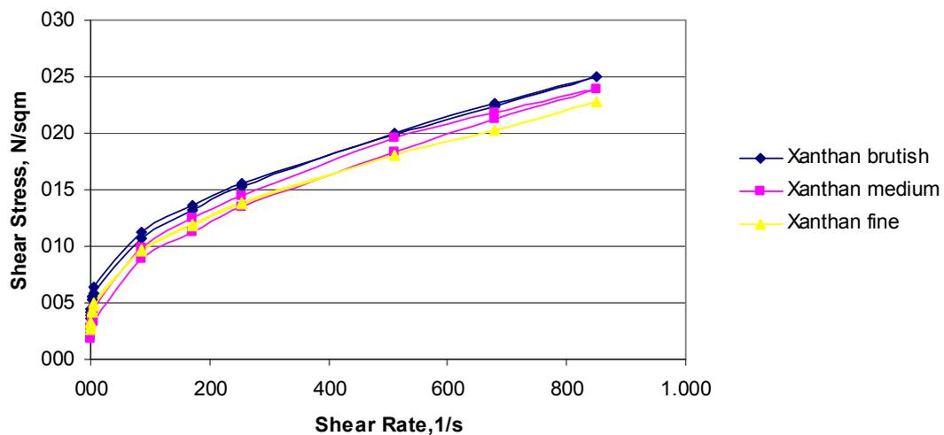
**Fig. 11.** The comparison of flow curves at different Xanthan gum granulation at 10% crude oil contamination.
