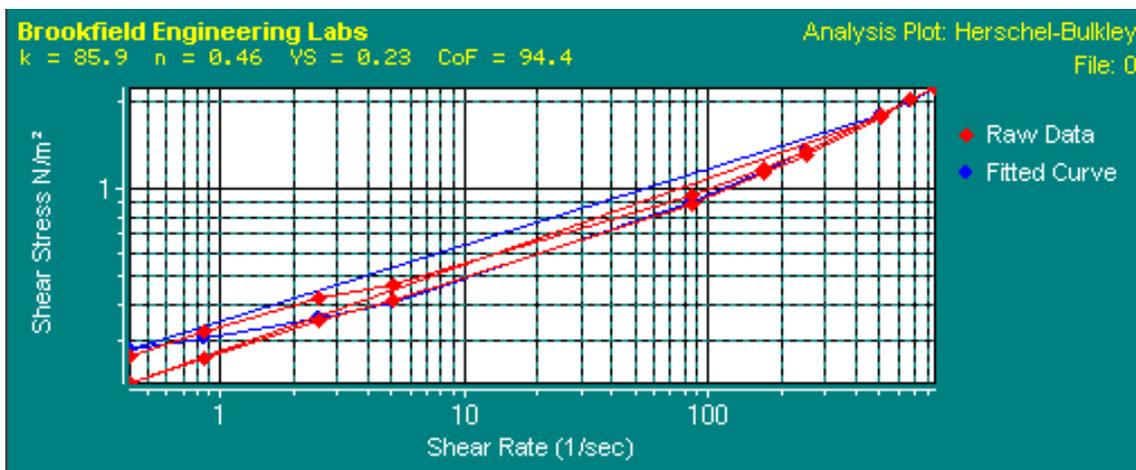
**Fig. 4.** The fitted and the experimental flow curves of an aqueous dispersion of fine Xanthan gum
