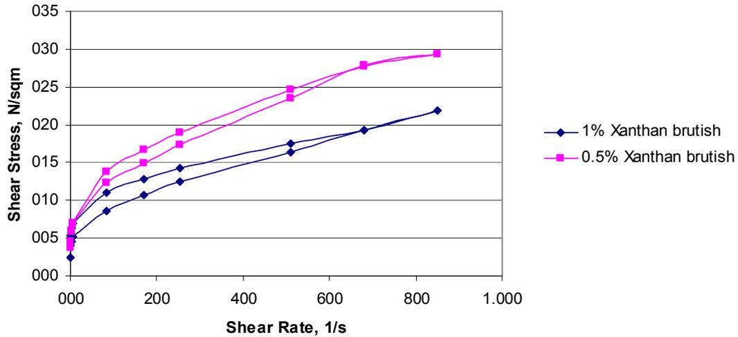
**Fig. 10.** The comparison of flow curves at different Xanthan gum concentrations at 50% crude oil contamination.
