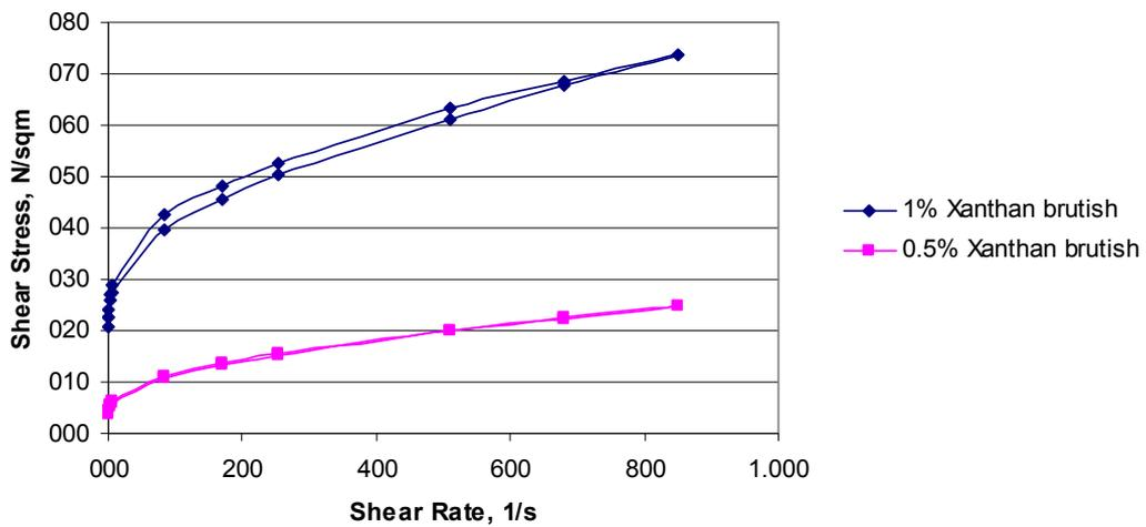
Fig. 9. The comparison of flow curves at different Xanthan gum concentrations at 10% crude oil contamination.
