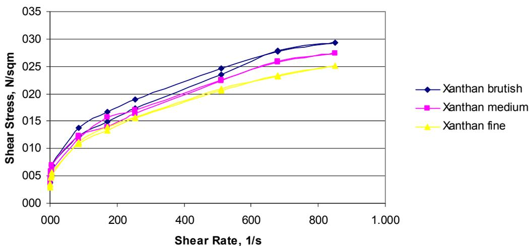
Fig. 12. The comparison of flow curves at different Xanthan gum granulation at 50% crude oil contamination.
