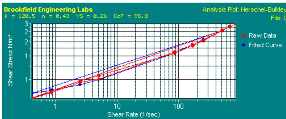
**Fig. 5.** The fitted and the experimental flow curves of an aqueous dispersion of fine Xanthan gum contaminated with 50%wt crude oil.
