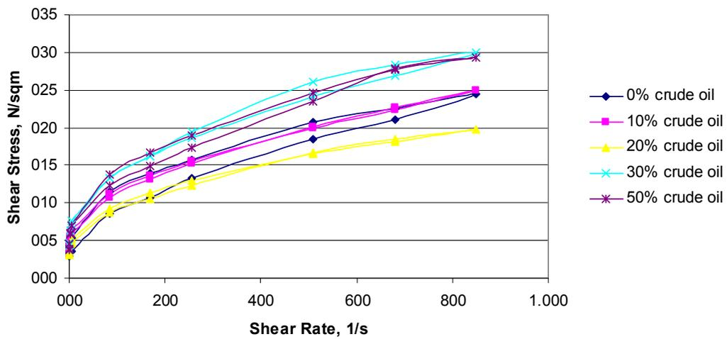
Fig. 7. The flow curves for 0.5% brutish Xanthan gum aqueous dispersion contaminated with crude oil.
