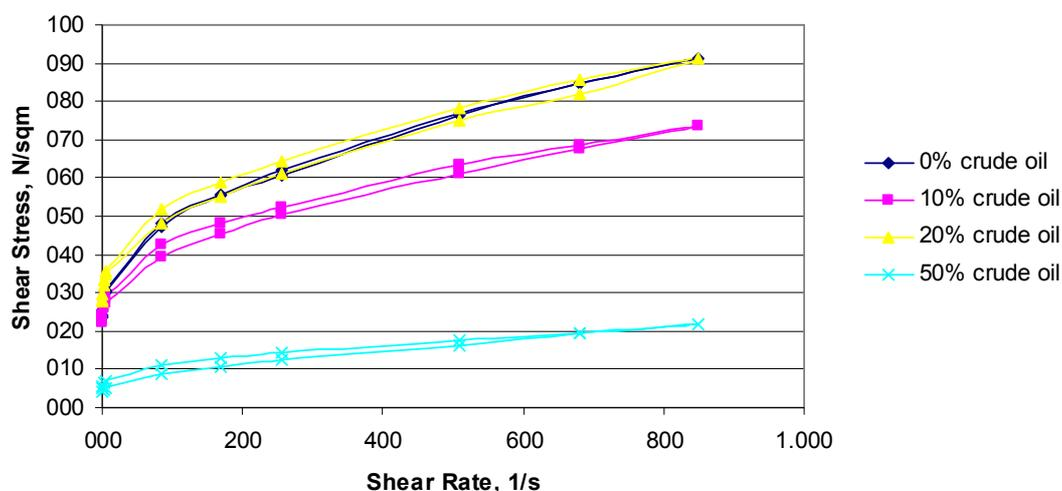
**Fig. 6.** The flow curves for 1% brutish Xanthan gum aqueous dispersion contaminated with crude oil.
