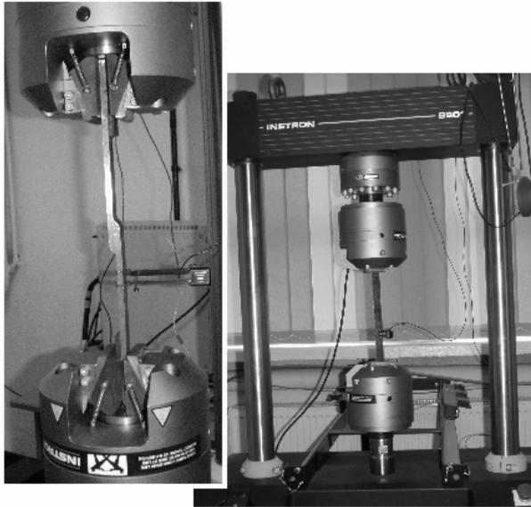
Fig. 3. Fatigue testing model
