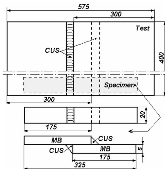
**Fig. 1.** Configuration and dimensions of the specimens and test-plates
