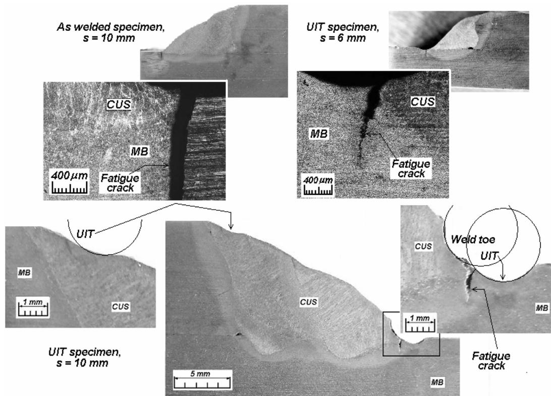
**Fig. 6.** Fatigue failure initiation areas on the fillet welded lap joints between steel plates
