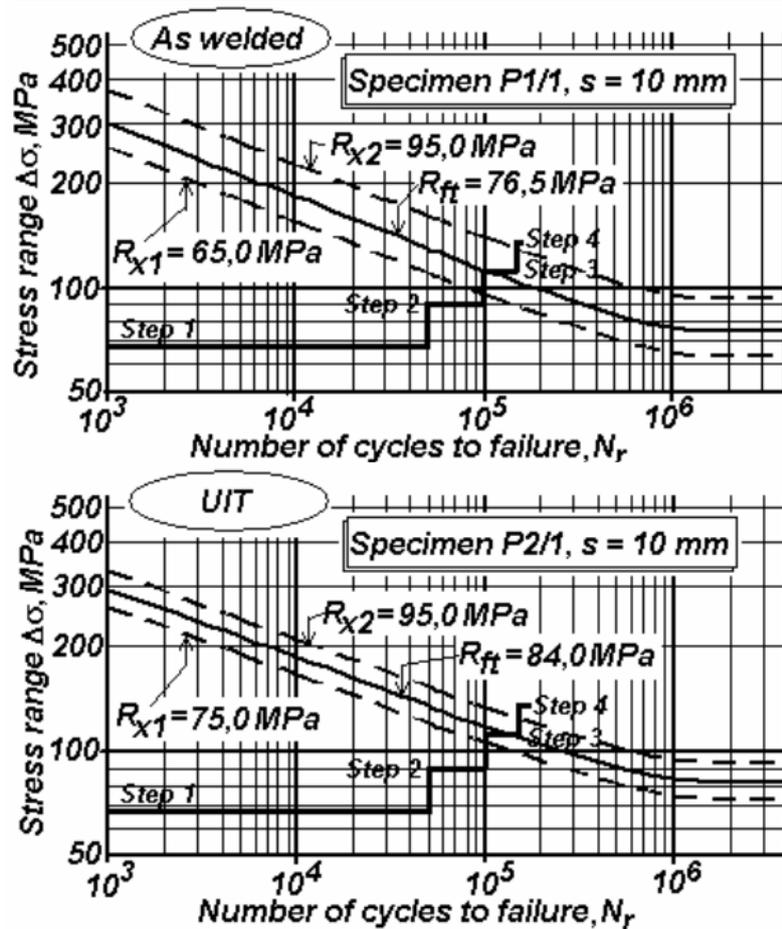
Fig. 5. Testing specimens P1 and P2,  $s = 10 \text{ mm}$  using the Locati method
