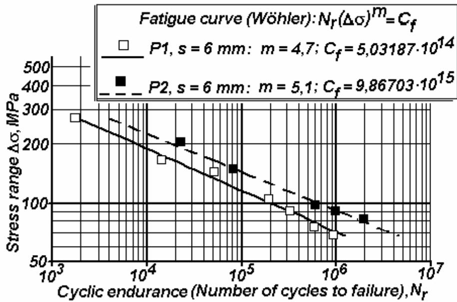
Fig. 4. Experimentally determined Fatigue curve (Wöhler)
