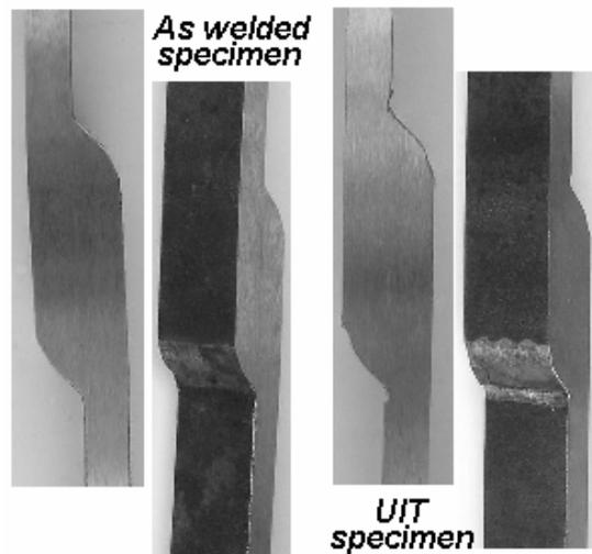
**Fig. 2.** Specimens ready for undergoing fatigue tests
