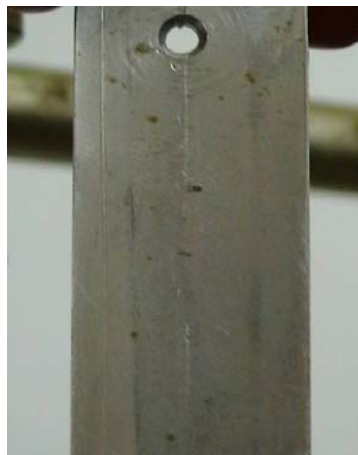
Fig. 4. Specimen of AISI 316L covered with shampoo film at 50°C after 3h30min.
