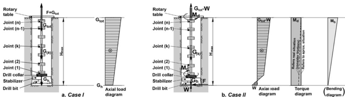
**Fig. 2.** The load and stress diagrams for the drill stem in both specific loading cases
