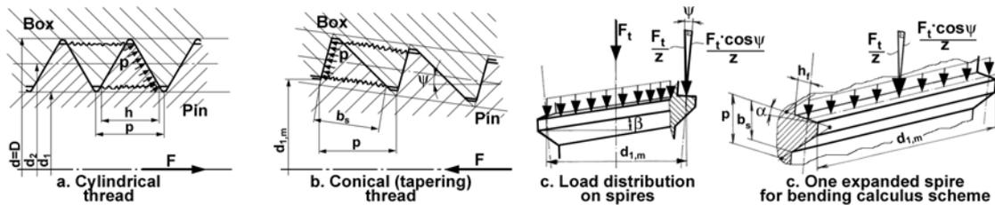
**Fig. 3.** The necessary calculus schemes for pin and box thread verifications
