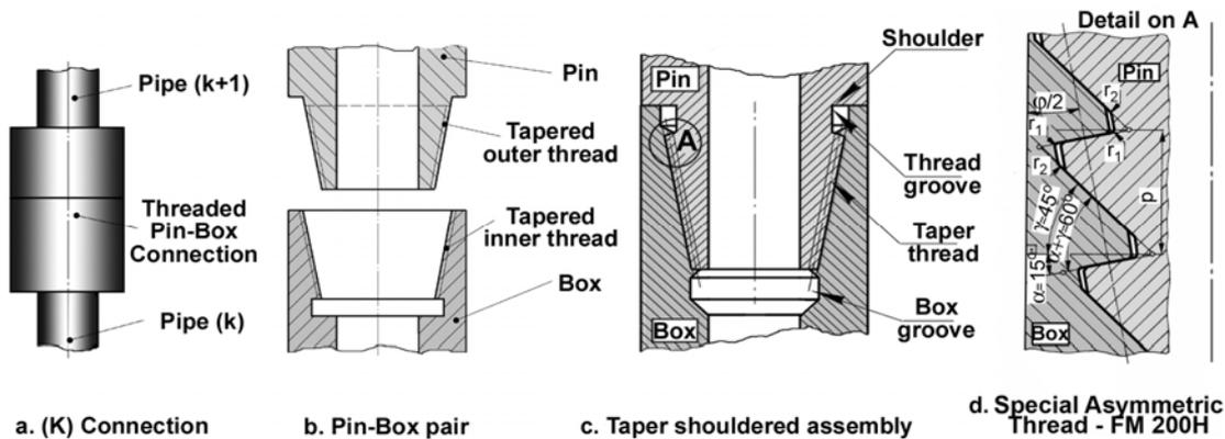
**Fig. 1.** Constructive and dimensional particularization of the threaded pin-box connection when used for large diameter drilling stem
