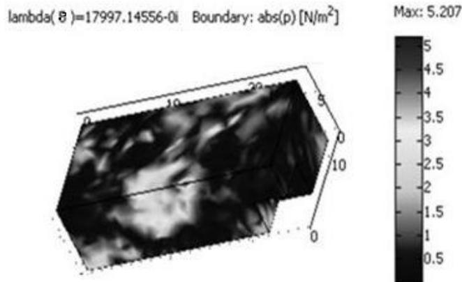
**Fig.3.** Distribution of absolute pressure  $abs(p)$  on boundary for Eigen frequency of 21.36 Hz; *sound hard boundary (wall)*, boundary condition for all boundaries.
