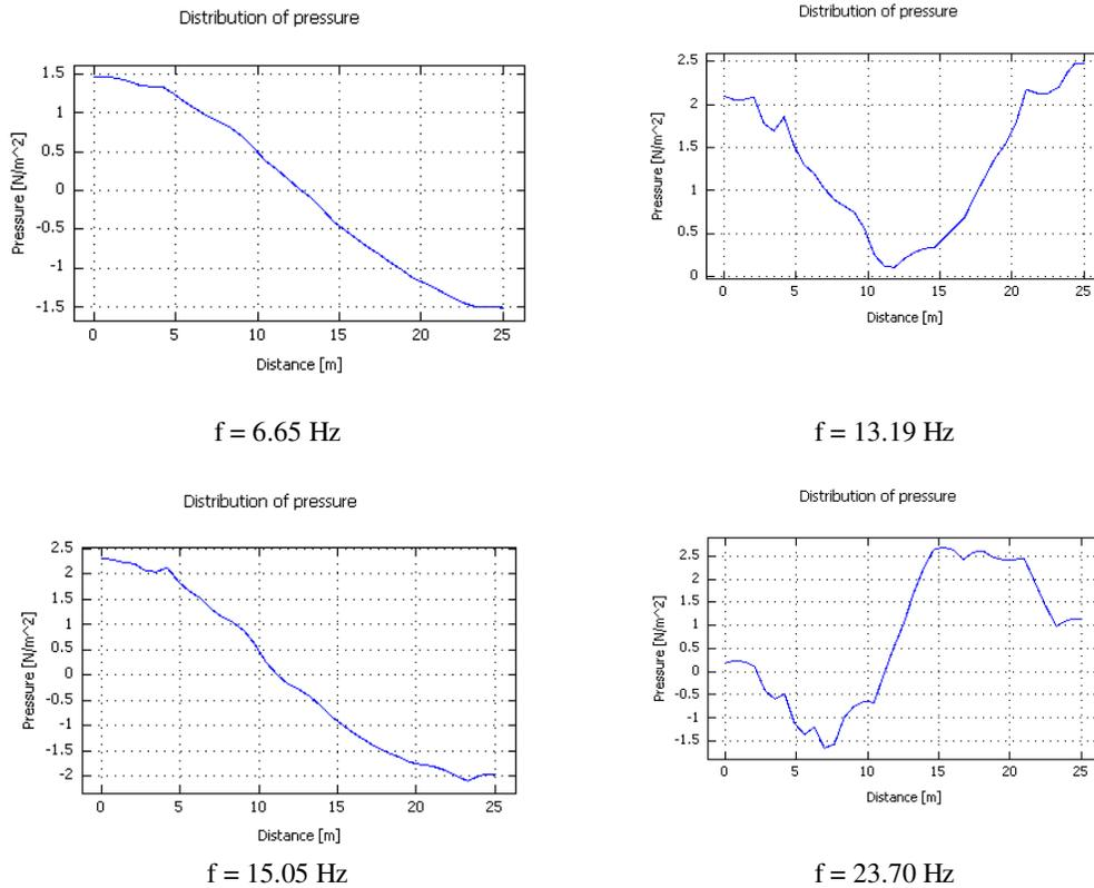
**Fig.2.** Distribution of acoustic pressure on the edge of the pumping room.
