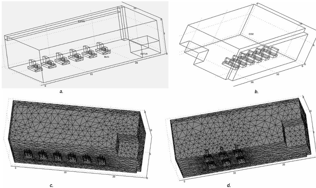
**Fig.1.** The model of pumping room: a) geometry 3D; b) compound object obtained by removing of office and pumping groups [8]; c) the model with mesh of finite elements in the case of six pumps inline; d) the model in the case of six grouped pumps.
