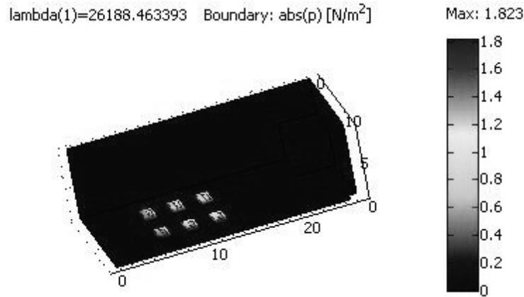
**Fig.4.** Distribution of absolute pressure  $abs(p)$  on boundary for Eigen frequency of 25.75 Hz; *sound soft boundary (wall)*, boundary condition for boundaries of the pumping room.
