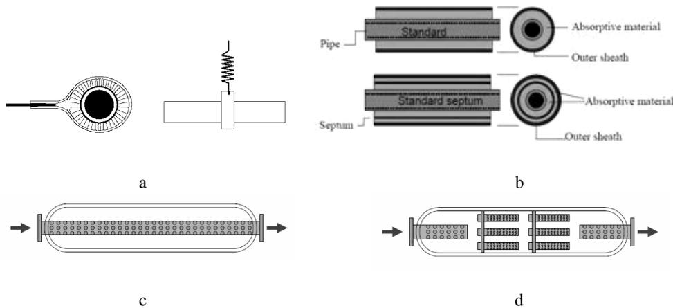
**Fig. 6.** Methods used in reduction of noise: a) elastic pipe hangers; b) cover absorptive material: standard; sandwiched septum layer; c) inlet pipe perforated with many small holes; d) multiple expansion chambers.
