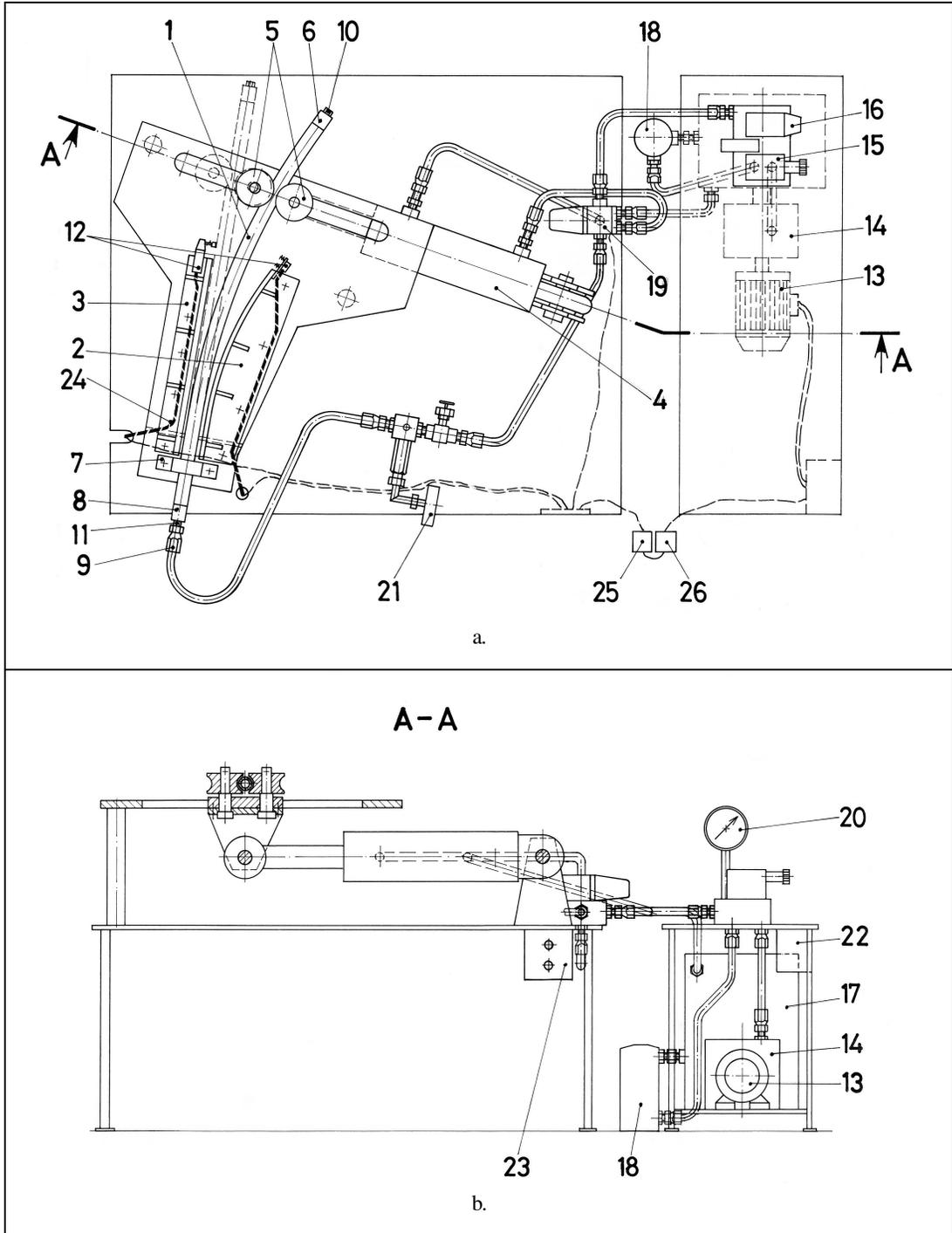
**Fig. 3.** The stand used for tests to bending with internal pressure:
