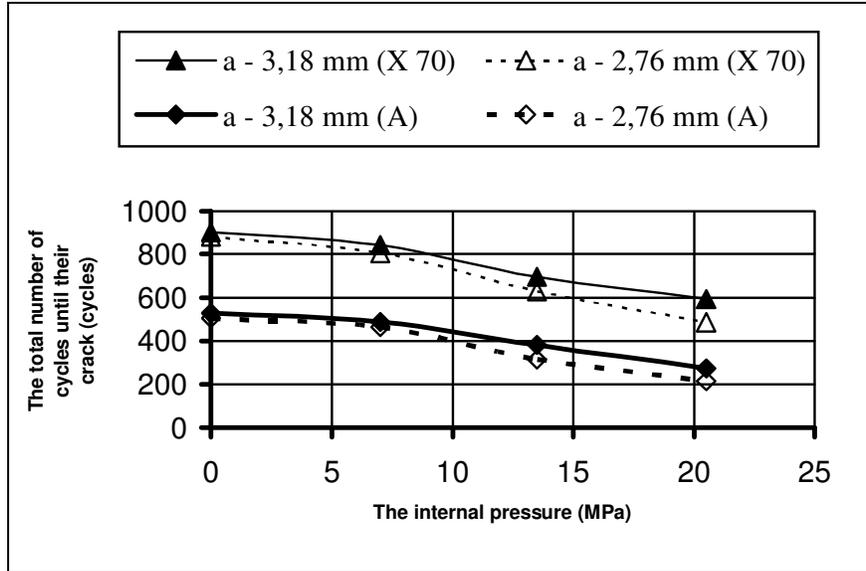
Fig. 4. The influence of the wall thickness and the material of the coiled tubing on the total number of cycles until cracking.
