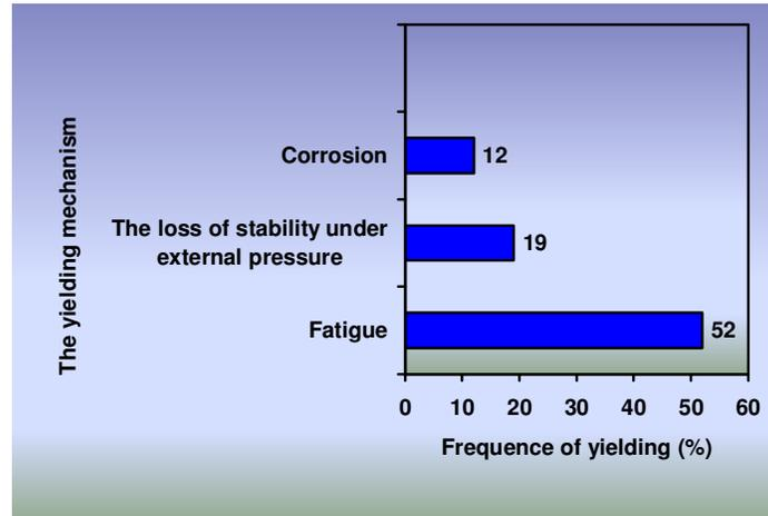
Fig. 2. The frequency of the coiled tubing yielding mechanisms [5].
