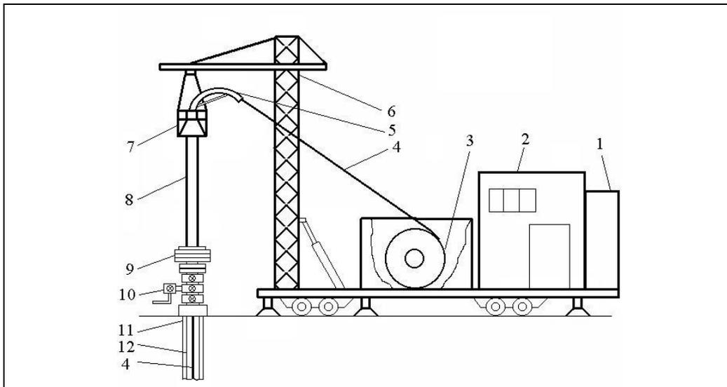
**Fig. 1.** The coiled tubing unit. 1 – pump room; 2 – control room; 3 – coiled tubing reel; 4 – coiled tubing; 5 – guiding arch („goose neck”); 6 – mast; 7 – injector head; 8 – lubricator; 9 – BOP stack; 10 – well head; 11 – casing; 12 – production tubing.
