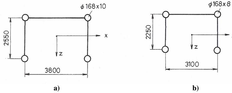
Fig. 2. MU200 cross sections
