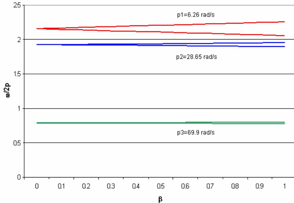
Fig. 3. Stability chart for the MU200 mast
