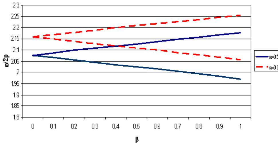
Fig. 4. Influence of the  $\alpha$  parameter on the stability chart for the MU200 mast
