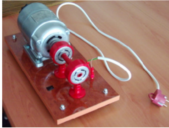
Fig.1 Permanent magnet bearing built in the Laboratory of Electrical Machines
