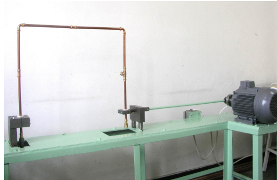
Fig. 1. Stand conceived for the vibration resistance test under bending loads of the copper pipes joints
