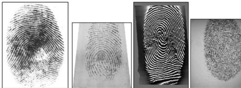
Fig. 1 Fingerprint images acquired with different optical scanners
