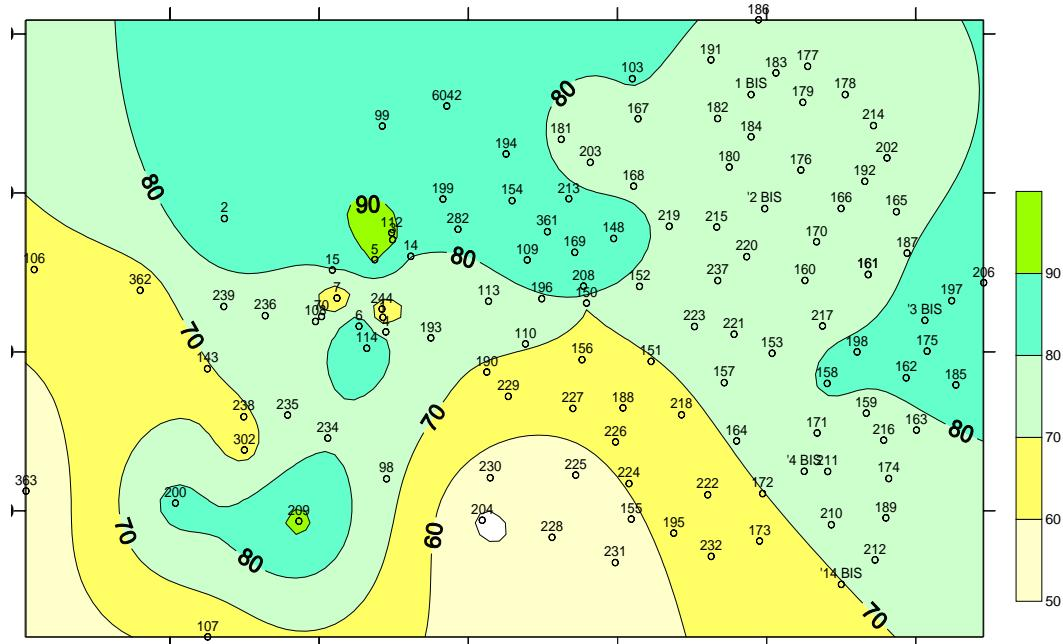
**Fig. 2.** Gas isosaturation map at Bg (IX-X)+X+XI+XII.
