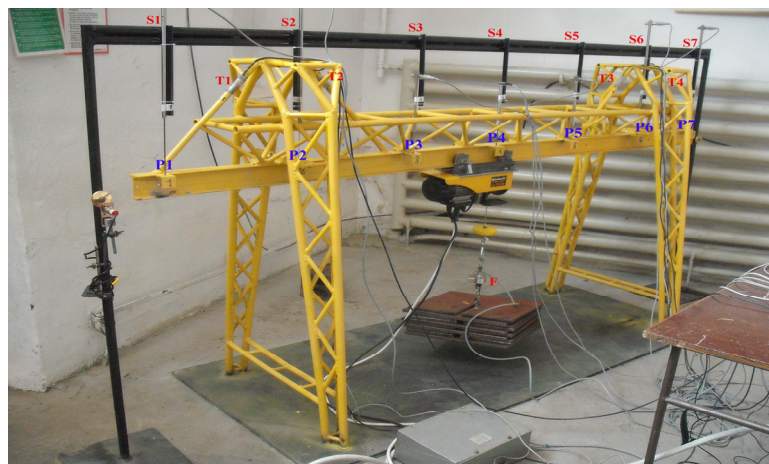
Fig. 6. Mounting scheme for deflections measuring
