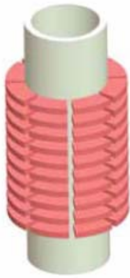
Fig. 1. The distribution of grapples around the casing surface
