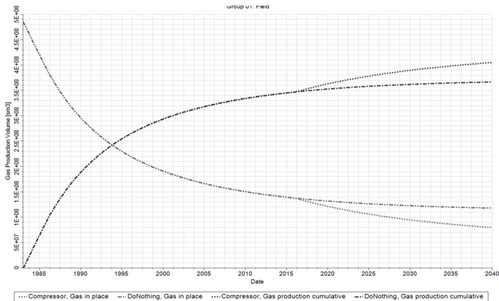
Fig. 11. Forecast comparison for the no further action against compressor simulations
