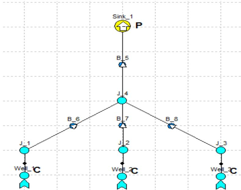
Fig. 5. PIPESIM model of the field's surface network
