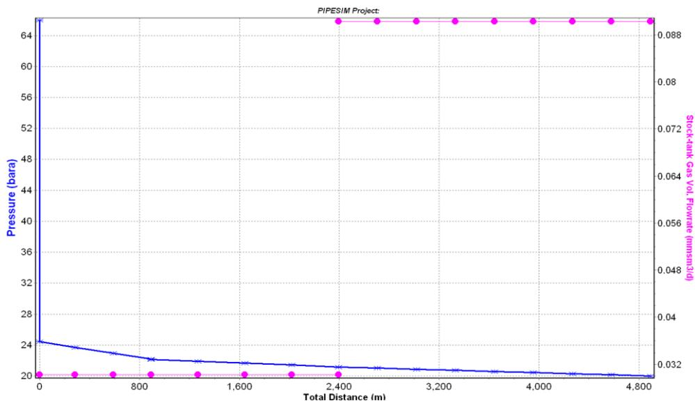
Fig. 6. Pressure–Flowrate (dotted line) against distance profile along Well\_2 (P2)–J2–B7–J4–B5–Sink1
