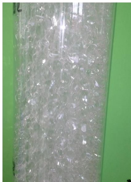
Fig.4. Detail presenting the foaming inside the testing installation
