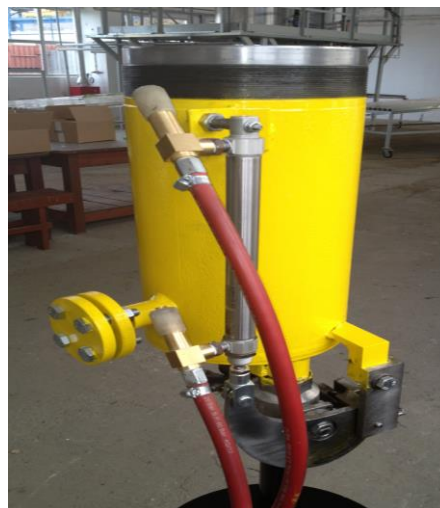
Fig.2. Automated launcher for solid biodegradable foaming sticks
