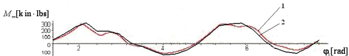
**Fig. 2.** The variation on a cinematic cycle of the motor moment at the cranks shaft for the pumping unit with which is equipped the well *Colibași 256* (curve 1 corresponds to the measurements results and curve 2 to the simulation results)
