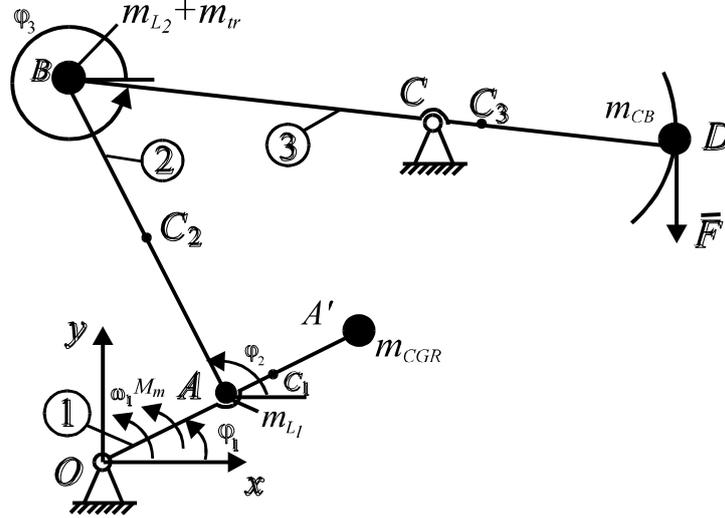
Fig. 1. Cinematic scheme of a pumping unit mechanism with conventional type geometry
