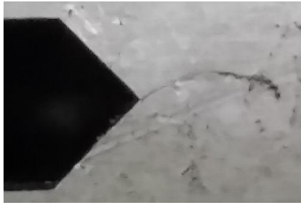
Fig. 5. Fore cracked specimen
