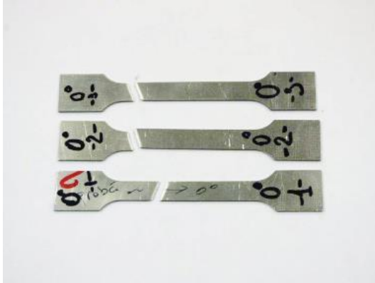
Fig. 1. Sample of the specimens used for traction test
