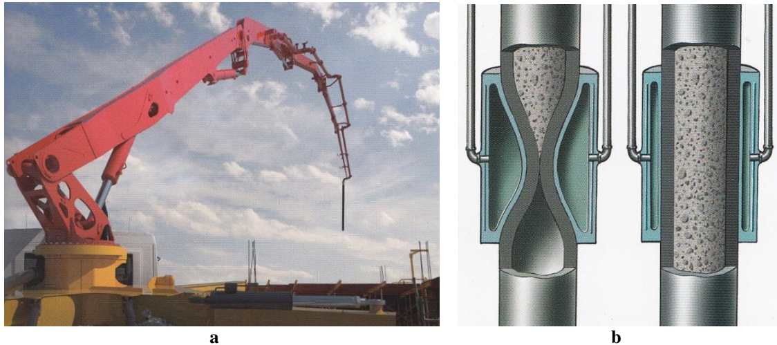
Fig. 1. The holding arm of concrete pump (a) with the hose end (b).
