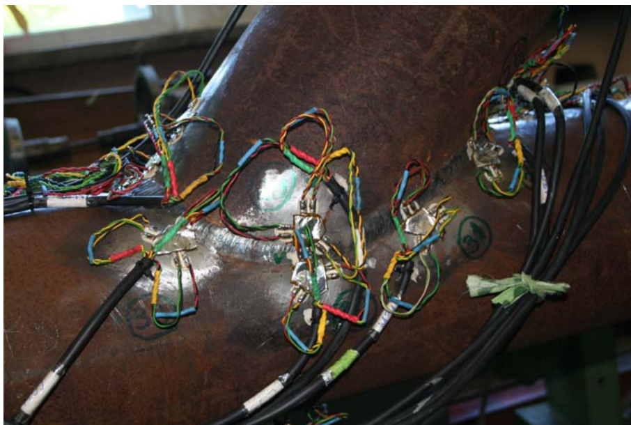
Fig. 6. Detail of the strain gauges layout, bottom view
